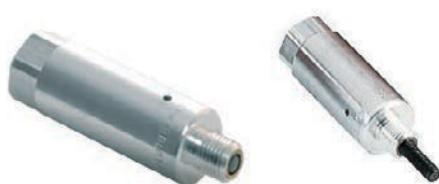
The Mini Mights offer the same friction free performance as ControlAir's larger sized diaphragm air cylinders. Mini Might are based on the unique rolling diaphragm principle that virtually eliminates friction. The fact that there is no stiction or blow-by of any kind permits uncompromising accuracy and repeatability.
