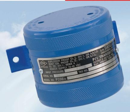
ControlAir's P200 P/I transducer represents outstanding value in pneumatic to current technology. All solid state circuitry converts standard 3-15 or 6-30 psig instrument air into 4-20 mA output with uncompromising accuracy and durability.
