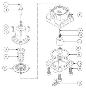
All items marked with an asterisk (\*) will be included in the repair kit. Other parts may be ordered separately by specifying the item number, part name, and the part number of the regulator for which the parts are intended.
